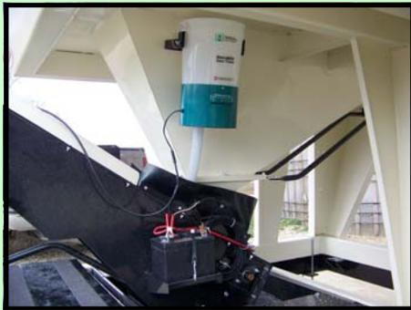
The "Low RPM/High Torque" motor & gearbox, combined with the adjustable slide gate, provides the accuracy of both systems.
