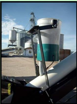
Model mounts to dispense product directly into hopper or conveyor. Can be wired direct to conveyor switch or separate 60' wiring harness.
