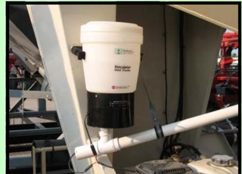
Auger Mount is complete with hanger brackets, mounting rails & wiring system. Special 2-way wiring powers both treater & auger. Discharge spout directs product onto "flowing" seed.
